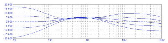
The fourth shows the bass and treble being adjusted while the mid band is at full cut. The mid band may not seem to be having much effect but the ear is so sensitive in this frequency range that a little goes a long way.
