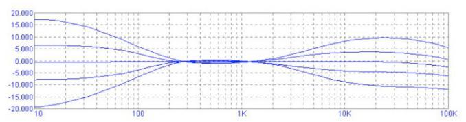
The third shows the bass and treble being adjusted while the mid band is set at full boost.
