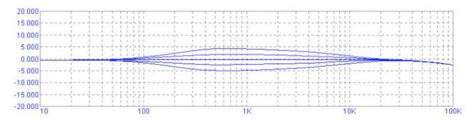
The second shows the bass and treble being adjusted while the mid band is left flat.
